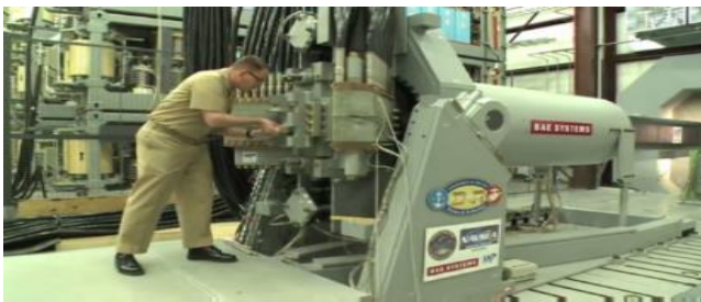
Figure 2 Full-scale laboratory testing of an EM Gun
